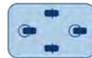
Wheel arrangement A: 2 swivel castors and 2 fixed castors, arranged in a rhomboidal position
